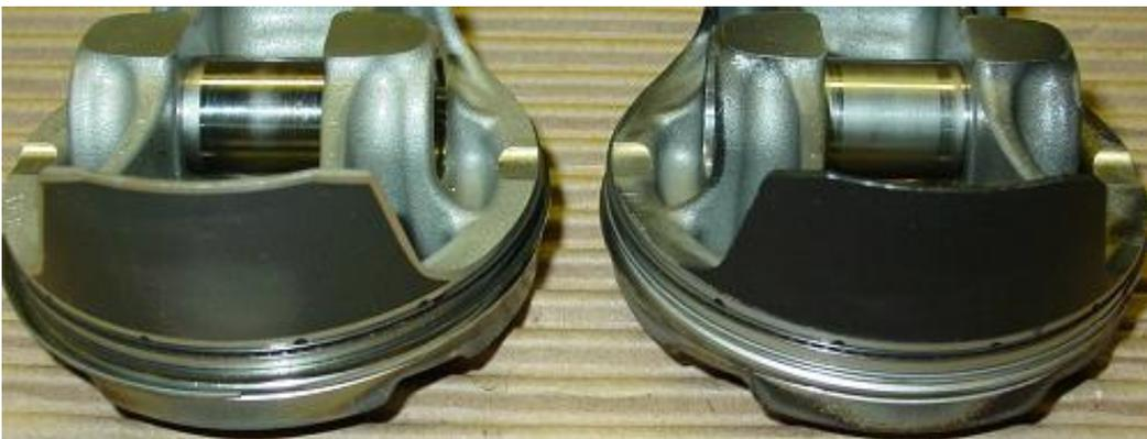
Figure 4 – APC™ engine (right) has less wear on wrist pins.
