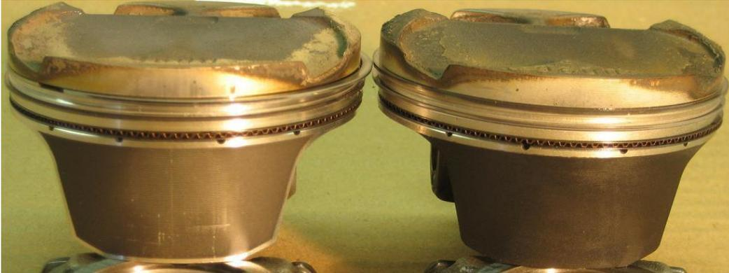
Figure 2 - Stock coating (left) smaller **skirt** contact pattern (bad for oil film) and scratches. Full skirt contact on APC™ piston means **better oil film and lower friction**. Stock coated piston has larger contact area and more wear on the **top land**. The APC™ pistons also had a thermal barrier crown coating.
