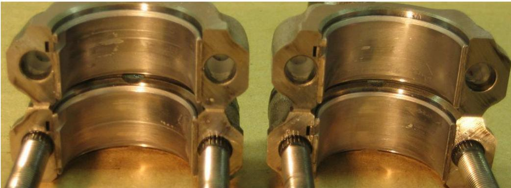
Figure 3 - APC™ engine (right) has less distress on bearings.
