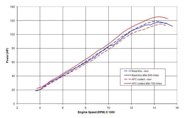
Figure 5 – Same dyno curves as Figure 1, but shown in engine RPM domain.
