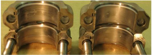
Figure 3 - APC<sup>™</sup> engine (right) has less distress on bearings.
