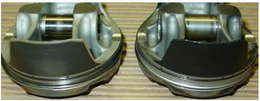
Figure 4 – APC<sup>™</sup> engine (right) has less wear on wrist pins.
