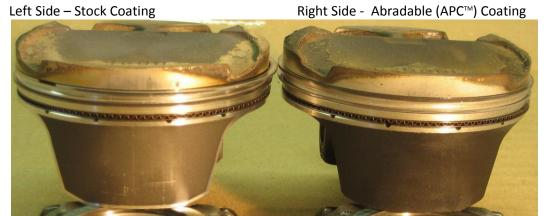
Figure 2 - Stock coating (left) smaller **skirt** contact pattern (bad for oil film) and scratches. Full skirt contact on APC<sup>™</sup> piston means **better oil film and lower friction**. Stock coated piston has larger contact area and more wear on the **top land**. The APC<sup>™</sup> pistons also had a thermal barrier crown coating.
